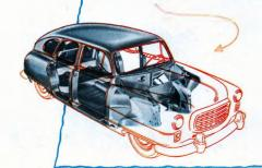
Different from all others, in Nash the entire frame and body, floor, roof, pillars are here built as a single, rigid, welded unit, squeak-free and rattle-proof Ithas 1½ to 2½ times the torsional strength of ordinary automobile construction. Gives newsafety, new economy, makes possible a safer, smoother ride. Stays new years longer, adds to resale value.
